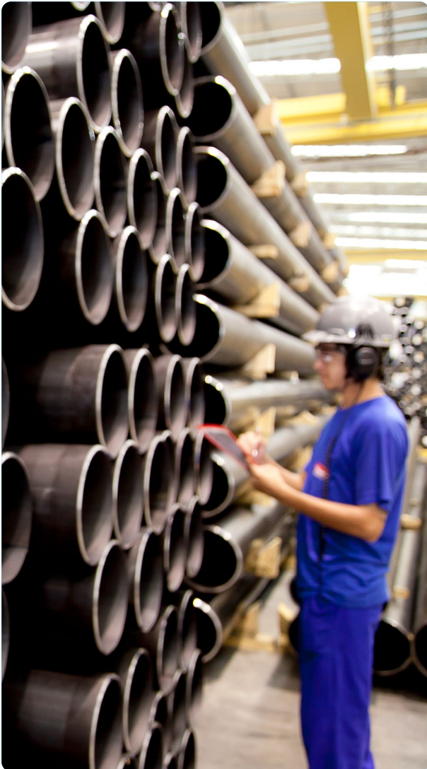
Grades: Reference values according to ASME B36 10 meters. Tubes are supplied in lengths from 6 to 14 meters.
